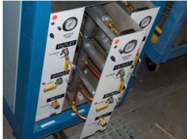
Figure 4: Heater units inserted in a rack. Heater assembly for Cavity 5-2 is shown partially removed to show the polyurethane slide.
