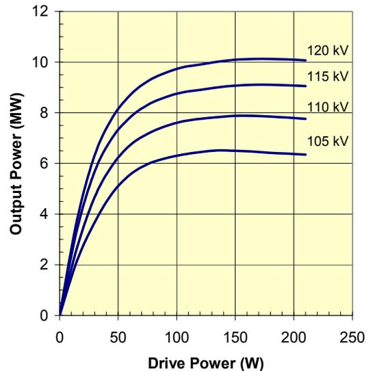
Figure 2: Output power versus drive power for several values of beam voltage.
