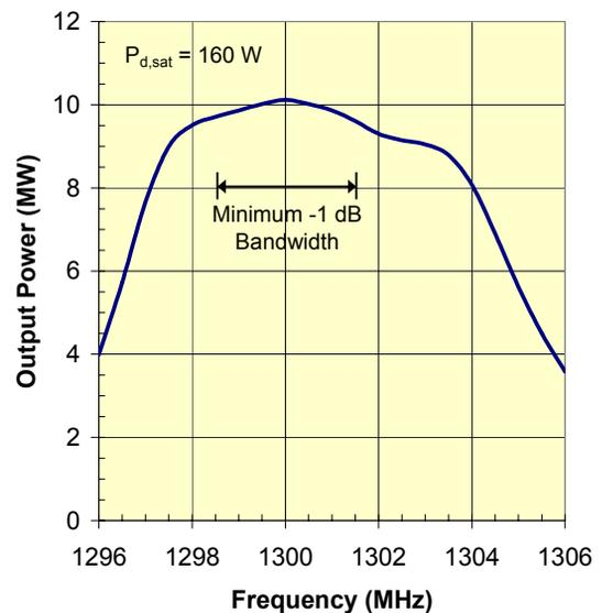
Figure 3: Saturated output power versus frequency.
