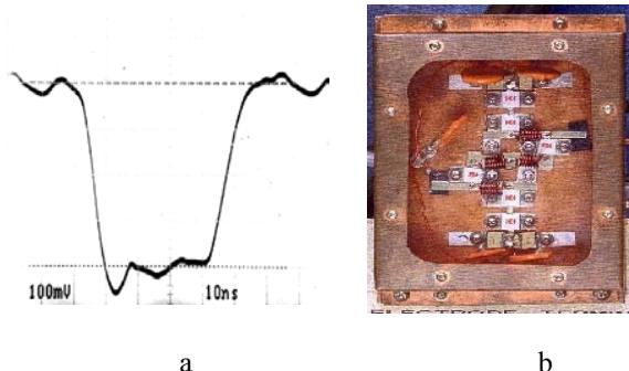
Figure 8: a-experimental waveform of 400 V 30 ns wide output pulse; b- 1250 W 125 Ohm RF load.
