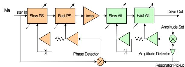
Figure 9: Simplified block diagram of 24.25 MHz rebuncher.
