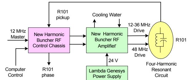
Figure 1: Four-harmonic buncher system block diagram.
