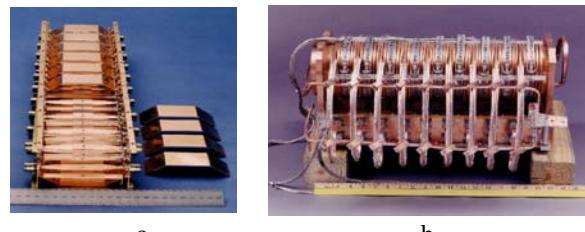
Figure 6: a-stripline deflection section, b-delay lines.
