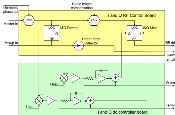
Figure 4: Simplified block diagram of the single frequency control channel.
