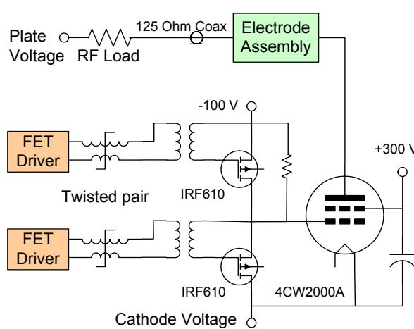
Figure 7: Simplified diagram of the RF driver. FET driver boards are DEI FPS-3N series fast power switch.
