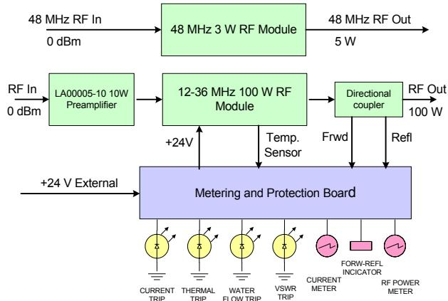
Figure 2: RF amplifier block diagram.
