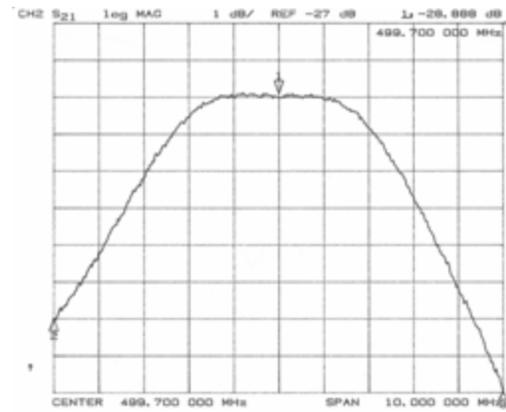
Figure 8: Typical S21 response of a tuned output cavity (scale 1 MHz/division; 1 dB/division)
