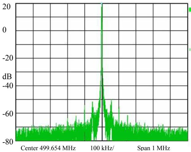
Figure 6: Spectrum of the output from the amplifier.
