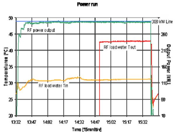
Figure 3: Plot of the output power over a two hour power run recorded on 23/11/04.
