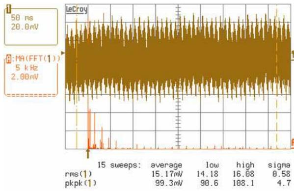
Figure 5: Output ripple of the amplifier under load.
