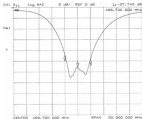
Figure 7. Typical S11 response of the input cavity (scale 5 MHz/division; 5 dB/division).
