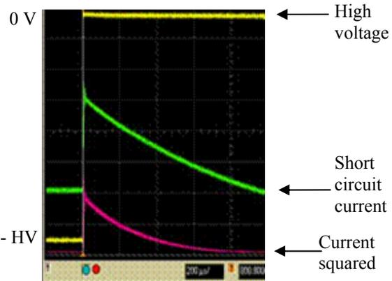
Figure 4: Plot of fault current during a simulated short circuit (Scale 5 kV/division; 20 A/division; 200  $\mu$ s/division).
