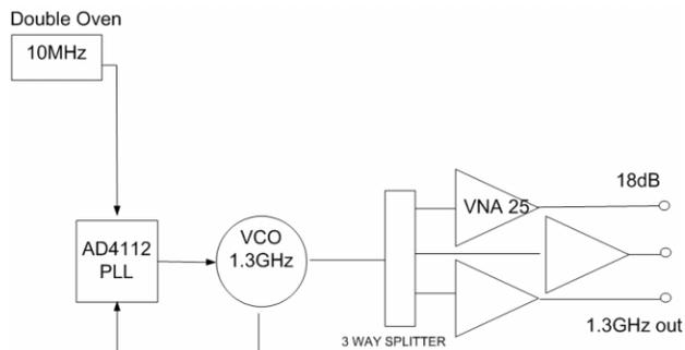
Figure 2: PLL and VCXO 1.3GHz Oscillator.
