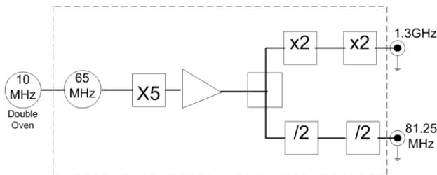
Figure 3: Multiplier based oscillator.
