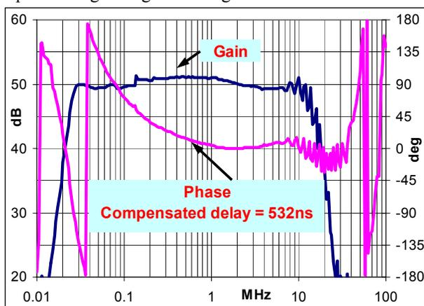
Figure 4: Input to grid transfer function.
