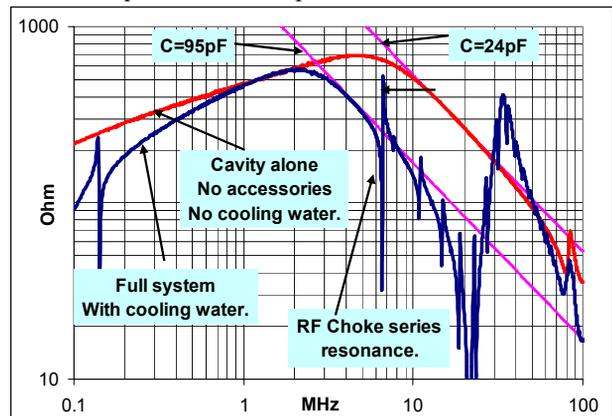
Figure 2: Cavity gap impedance.
