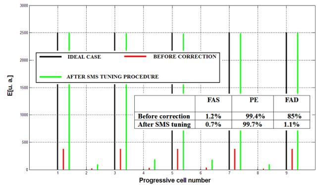
Figure 2: Field equalization for  $\pi/2$  mode ( $\delta f = \pm 4MHz$ ) of 9 cavities.
