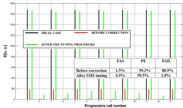
Figure 3: Field equalization for  $\pi/2$  mode ( $\delta f = \pm 4MHz$ ) of 13 cavities.
