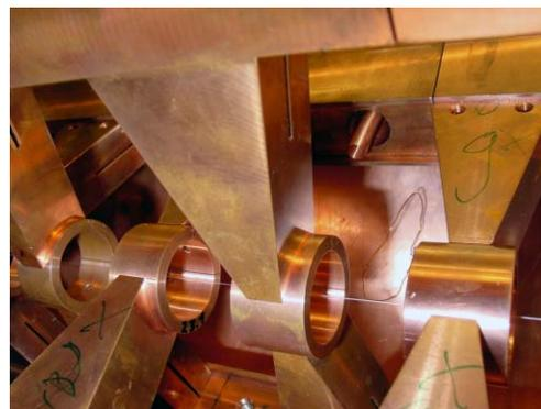
Figure 2: Capacitive coupling through one girder between two stems in the same plane
