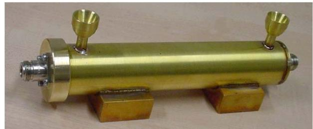
Figure 5: Coaxial measuring line for coolants.
