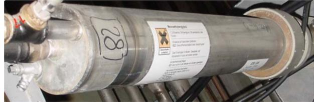
Figure 1: 100-kW, 500-MHz coaxial load for 30% glycol-water coolant. The load type was designed and build at DESY. Due to the usage of glycol the attenuation constant has been increased from about 17dB/m to 26dB/m @ 30°C coolant temperature. Thus it was feasible to make the design relative compact.
