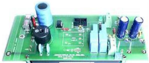
Figure 2: DC/DC converter board.
