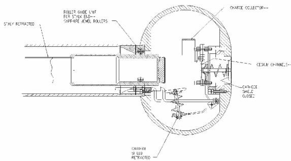
Figure 2: Detail of the inside of the ball cathode with the stalk retracted. The shield door is closed only during high voltage conditioning.
