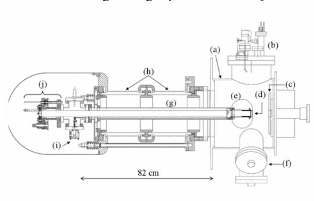
Figure 1: DC photocathode gun schematic. (a) vacuum chamber, (b) instrumentation, (c) anode, (d) photocathode, (e) ball cathode, (f) NEG pumps, (g) ball support tube, (h) ceramics, (i) shield door actuator mechanism, and (j) stalk retracting mechanism.
