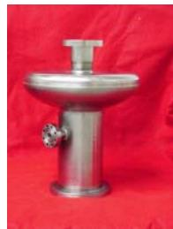
Figure 1: Photocathode cavity, the photocathode insert is shown in the right sketch
