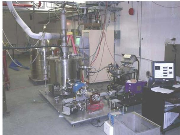
Figure 2a: Photograph of the beam transport system. The large cylinder in the background is the cryostat containing the cavity, the blue component in the middle is the focusing solenoid and the horizontal bar in the foreground supports optical elements to transport the laser beam to the cavity.
