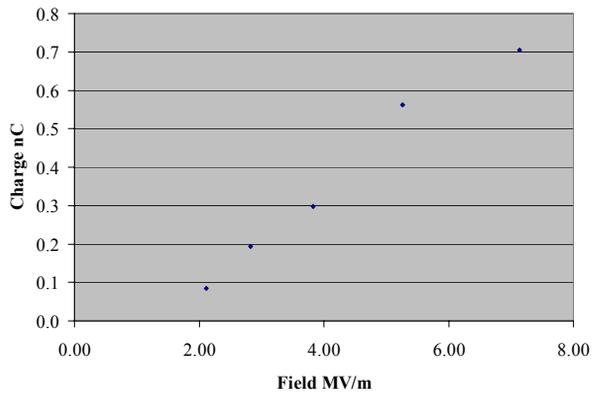
Figure 4: Charge vs cavity field for 3 mJ laser energy. The linear increase of charge at low fields is indicative of the presence of space charge effects. Onset of space charge free emission requires fields > 7 MV/m for this configuration .
