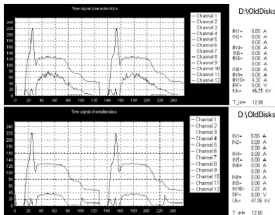
Figure 3: Oscillograms for the closed mode of magnetron gun operation. a) in the rising magnetic field; b) in the falling magnetic field.
