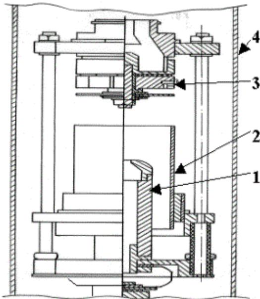
Figure 1: Schematic of the experimental setup. 1 - cathode, 2 - anode, 3 - Faraday cup, 4 - vacuum chamber.
