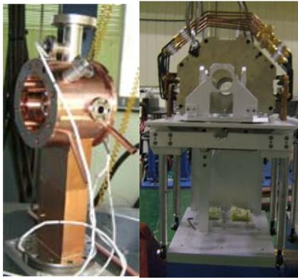
Figure 1. The RF Photo-Cathode (PC) Gun is brazed in the PAL (left) and the solenoid magnet and the stand is fabricated (right).
