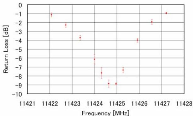
Figure 8: Return loss at the gun cavity.
