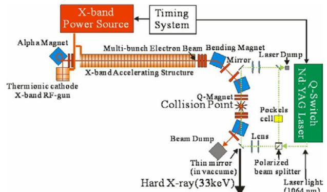
Figure 1: Beam line for a test of Compton scattering.
