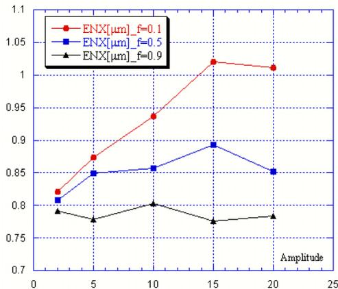
Figure 3: Projected horizontal emittance at the end of the linac versus the amplitude oscillations for frequencies of  $0.1 \text{ ps}^{-1}$  (red dots),  $0.5 \text{ ps}^{-1}$  (blue squares) and  $0.9 \text{ ps}^{-1}$  (black triangles).
