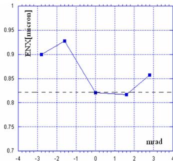
Figure 5: The projected emittance at the end of the linac versus crystal tilting angle. The dashed line is the reference emittance value for a perfectly aligned crystal.
