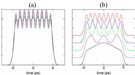
Figure 2: Frame (a): Intensity temporal profiles with different amplitude oscillations in the flat-top for a fixed frequency of  $0.9 \text{ ps}^{-1}$ . Frame (b): Intensity temporal profiles with different oscillation frequencies on the plateau for a fixed amplitude of 20%.
