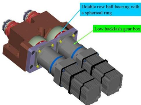
Figure 2: Double cam-shaft mover assembly.
