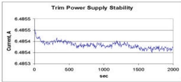
Figure 3: Bipolar trim power supply test.
