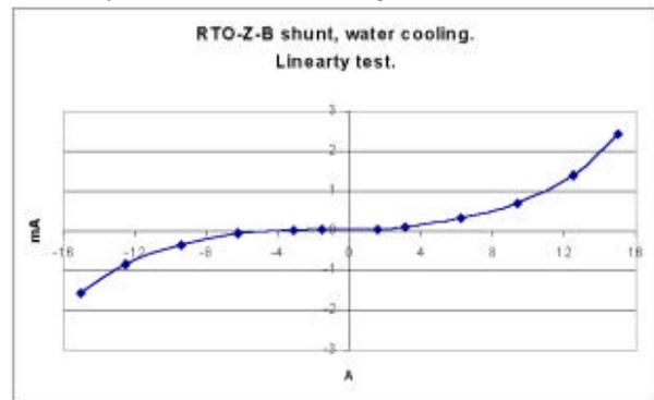
Figure 2: Unipolar 12A power supply nonlinearity.
