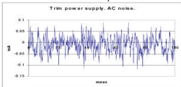
Figure 5: Trim power supply noise measured in the pass band 1Hz – 1kHz.
