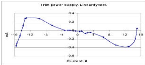
Figure 4: Difference between measured current and its linear fit.
