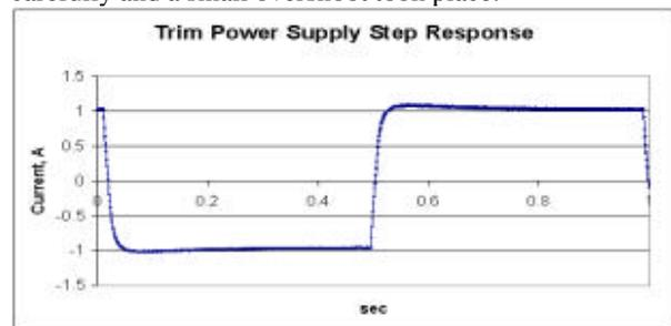
Figure 6: Bipolar power supply step response, crossing zero current.
