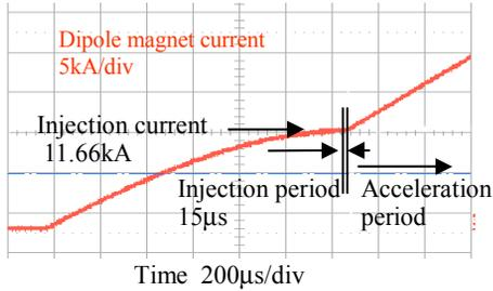
Figure 7: Measured time-dependent excitation curve of the dipole magnet for injection and acceleration.
