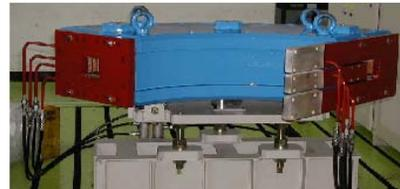
Figure 1: Dipole magnet (inductance is 2.9 $\mu$ H at low field, 1.5 $\mu$ H at high field (3T)).
