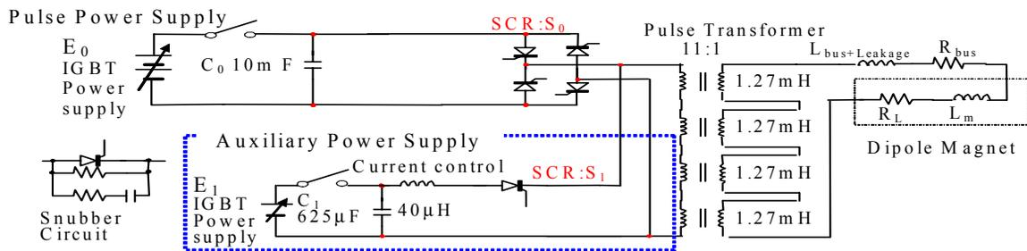
Figure 5: Pulse power supply for the acceleration and auxiliary power supply for injection.  $L_m$  2.9 $\mu$ H-1.5 $\mu$ H/magnet  $R_L$  27 $\mu$  $\Omega$ /magnet.
