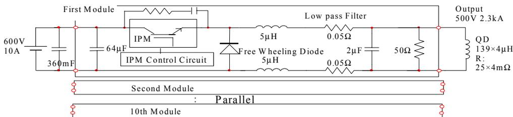
Figure 8: Circuit of the high frequency switch-mode power supply.
