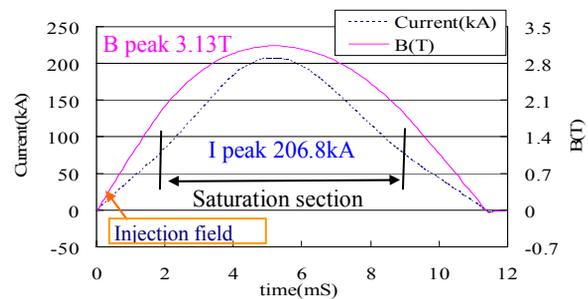
Figure 2: Measured time-dependent excitation curve.
