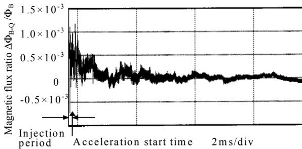
Figure 10: Simulation result for the tracking between the QD and dipole fields.
