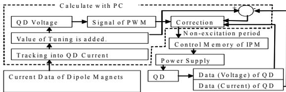
Figure 9: Control system of the switch-mode power supply.
