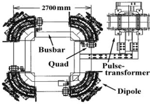
Figure 3: Layout of dipoles and quadrupoles. Tune is  $Q_x/Q_y=1.6/0.6$ .
