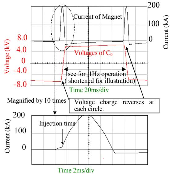
Figure 6: Operation of power supply.
