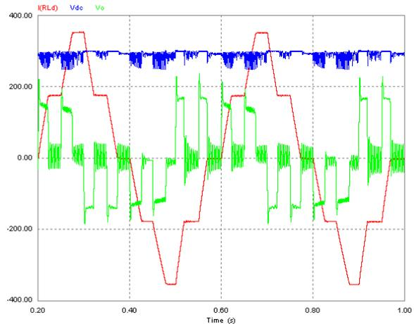
Figure 6: Simulation results of AC power supply, DC link voltage (300V), Load current (350App) and voltage (140V).
