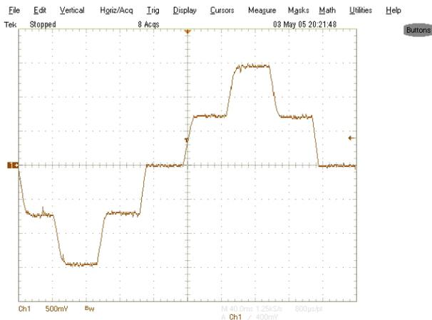
Figure 8: Actual load current of magnet.
