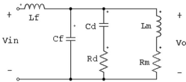
Figure 3: Output filter with magnet load.
