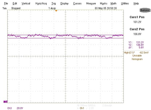
Figure 9: Fluctuation voltage of DC link.
