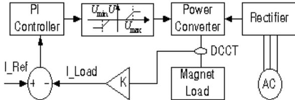
Figure 7: Control loop of DSP.
