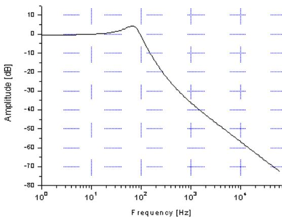
Figure 4: Amplitude responses of the designed filter, simulated by the PSPICE.
