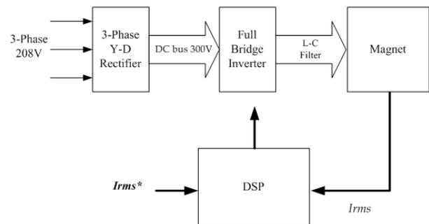
Figure 2: Block diagram of proposed AC power supply.
