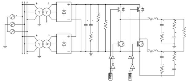
Figure 5: Model circuits of proposed AC power supply.
