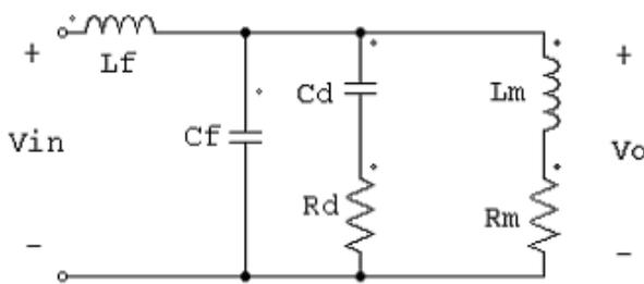
Figure 3: Output filter with magnet load.
