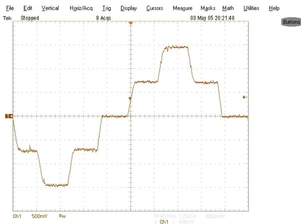
Figure 8: Actual load current of magnet.
