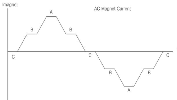
Figure 1: Required AC magnet current shape. A, B, C, D, E denotes each beamline.
