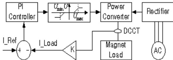
Figure 7: Control loop of DSP.
