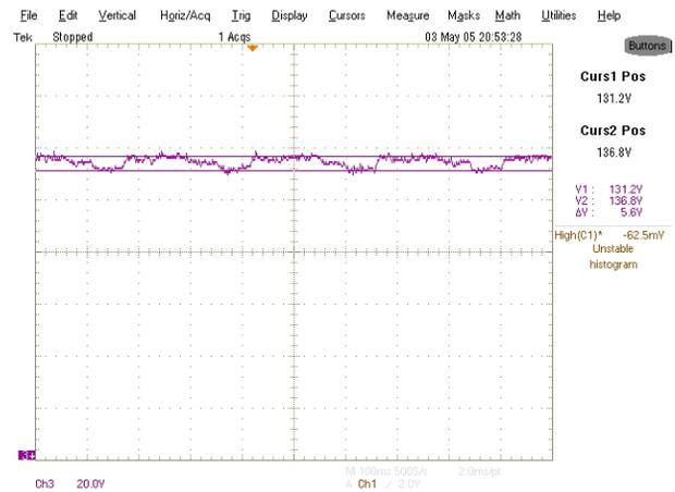
Figure 9: Fluctuation voltage of DC link.
