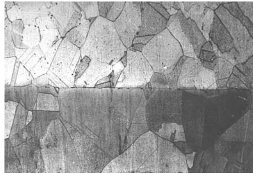
Figure 4: Effect of the diffusion temperature on the copper structure (x200).
