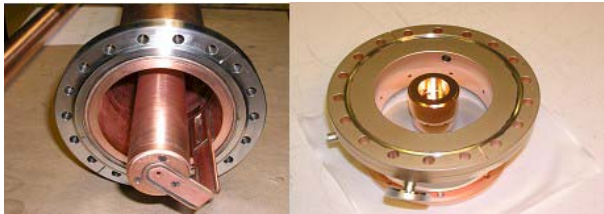
Figure 5: The coaxial loop coupler for the 201.25 MHz prototype cavity (left), ceramic window (right) is an integral part of the coupler.
