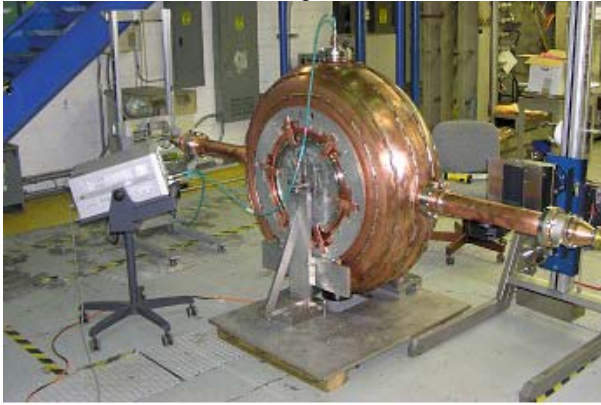
Figure 4: The 201.25 MHz prototype cavity with water cooling tubes (copper) welded onto the outer surface of the cavity. Two RF loop couplers were attached to the cavity for low power RF measurement of the frequency and coupling.
