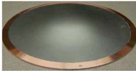
Figure 6: The first successful 0.38-mm thick and 420-mm diameter curved beryllium for the 201.25 MHz cavity. The beryllium foil is sandwiched (brazed) between two annular copper frames.
