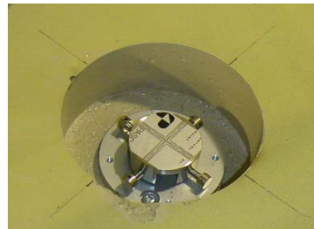
Figure 1: View of the beam line reference point. Watertight cover will be attached.
