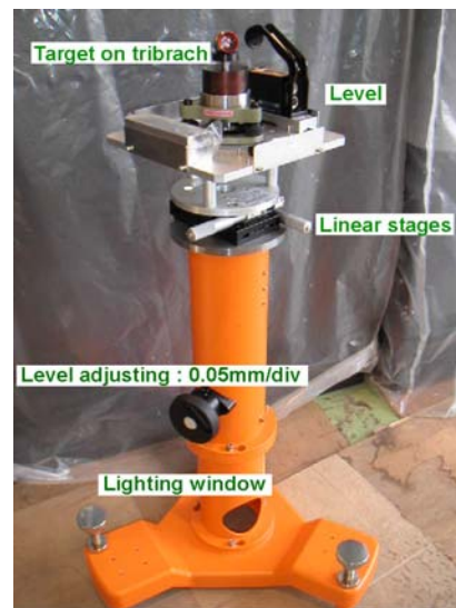
Figure 3: Alignment target mount. A fine (0.05mm/div) elevation stage is equipped in the lower mount. Linear stages and lower mount has a through hole to see the floor marking by NL.
