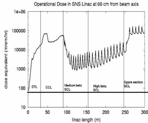
Figure 1: Dose at 60 cm distance from the Linac beam axis due to beam losses in normal operation [1]
