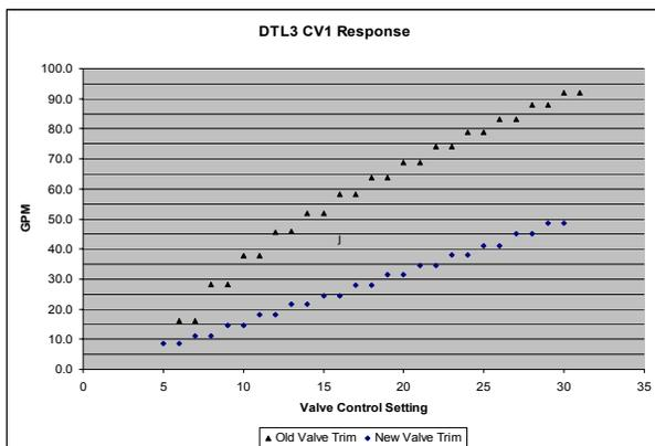
Figure 4: DTL3 RCCS CV-1 valve response.
