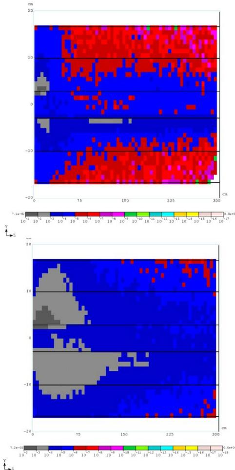
**Figure 3:** Longitudinal energy deposition in Gy/sec at 500 MeV (top) and 5 GeV (bottom) incident energy.
