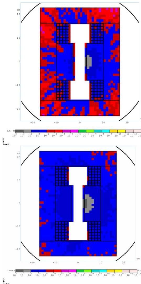
**Figure 5:** Residual radiation on contact after 30 days of operation and 1 day of cool down for 500 MeV (top) and 5 GeV (bottom) incident beam. These rates are consistent with surveyed activation.
