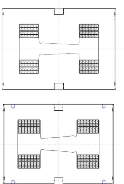
**Figure 1:** Booster magnet cross sections. Each magnet is approximately 13" high by 18" wide.
