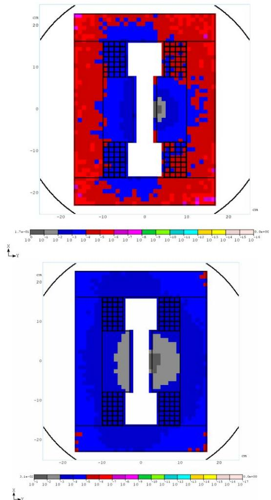
**Figure 4:** Cross sectional energy distribution, showing the energy deposited in the coil packs at 500 MeV (top) and 5 GeV (bottom) incident energy.
