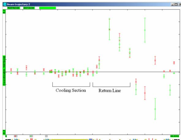
Figure 4 Example of trajectory deflection due to MI ramp. Full scale on y-axis is  $\pm 2$  cm.
