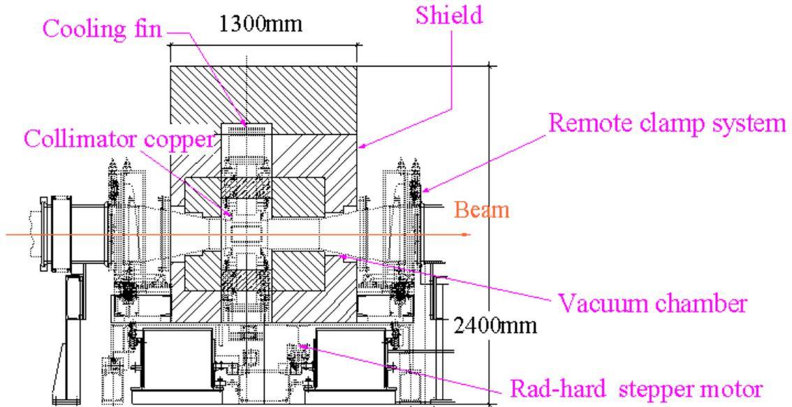
Figure 2: Schematic of J-PARC RCS collimator.
