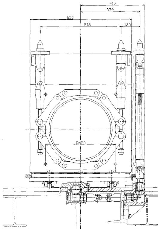
Figure 4: Schematic of the remote clamp system □
