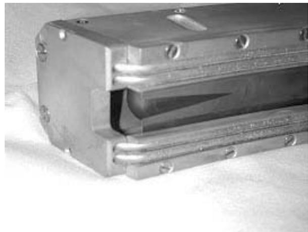
Figure 2: lateral view of the new water-cooled electrostatic deflector.
