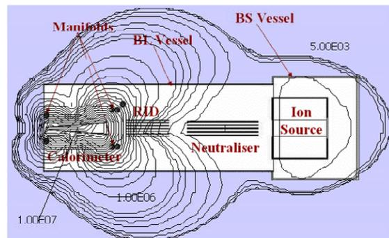
Fig. 4: Neutron flux ( $\text{n}/\text{cm}^2$ ) for an average current of 1 A.
