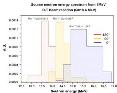
Fig. 2: D-T neutron spectrum.
