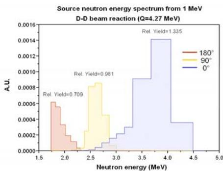
Fig. 1: D-D neutron spectrum.
