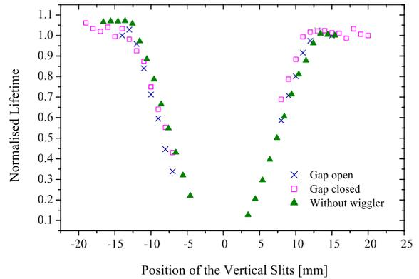
Figure 4: Effect of the wiggler on dynamic aperture.
