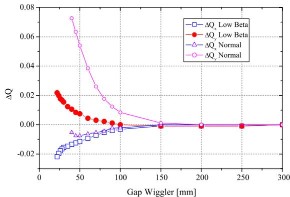
Figure 3: Measured tune shift at different wiggler gaps.
