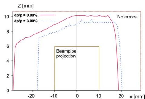
Figure 5: The storage ring dynamic aperture (ID).
