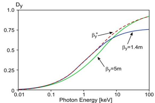
Figure 4: The normalized CANDLE brightness versus photon energy for various vertical beta.
