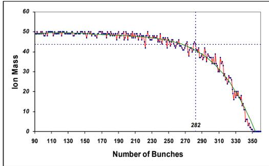
Figure 9: Number of unstable ions versus number of bunches in the ring.
