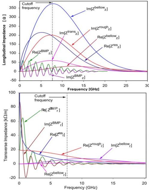
Figure 6: Longitudinal and transverse impedances of the ring caused by the walls resistivity, roughness, BPM's and transitions.
