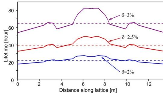
Figure 11: Touschek lifetime evolution along the lattice for various energy acceptances (solid lines).
