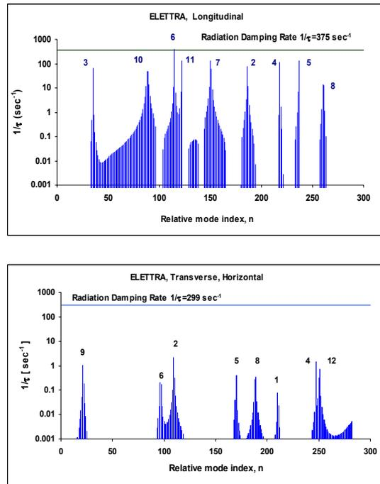
Figure 8: The longitudinal and transverse coupled bunch instabilities growing rate versus beam oscillation modes.
