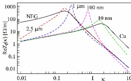
Figure 7: Real part of copper-NEG tube longitudinal impedance for various cover thickness.
