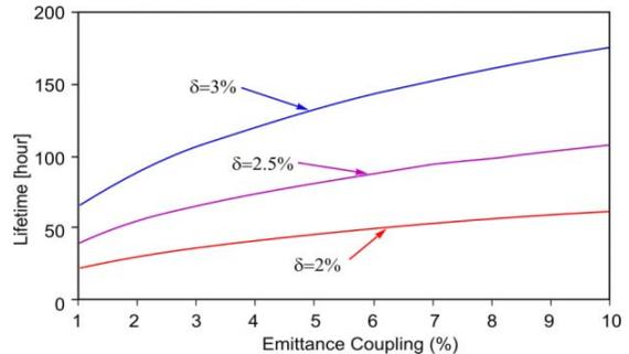
Figure 12: Averaged Touschek lifetime vs emittance coupling and energy acceptance.
