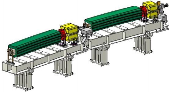
Figure 4: An SSRF booster cell Assembly.
