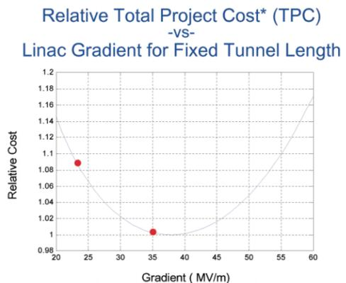
Fig. 1: Estimated Cost vs. gradient [5].
