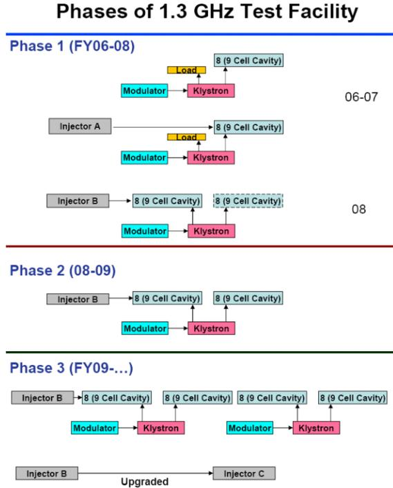
Figure 5: SMTF 3 steps for ILC module test.
