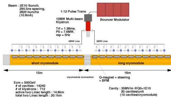
Figure 4: RF unit configuration of ILC main linac.
