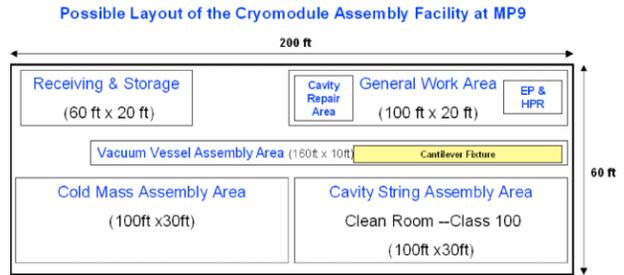
Figure 6: SMTF cryomodule assembly facility plan.
