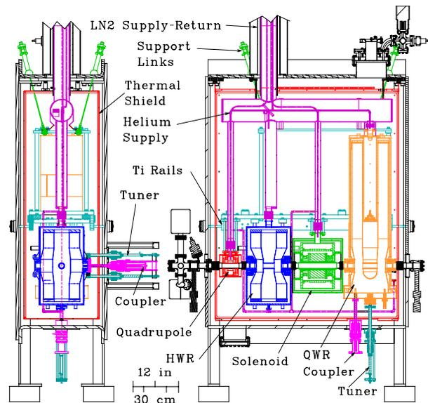
Figure 1. Sectional view of the prototype cryomodule.
