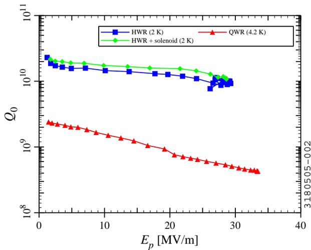
Figure 3. RF test results for the HWR, HWR in proximity to the solenoid, and QWR.
