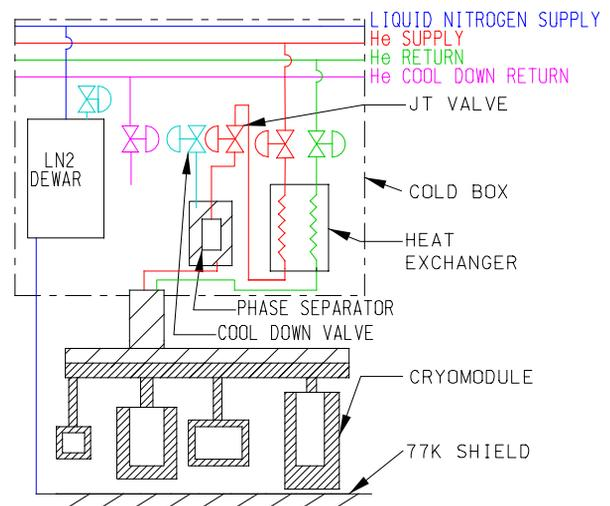
Figure 2. Schematic of cold box and prototype cryomodule.
