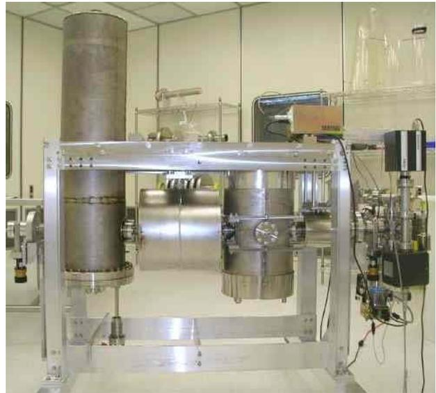
Figure 4. Cold mass assembly on titanium alignment rail inside the clean room. From left: QWR with RF coupler, solenoid with Nb shield, HWR with upper and lower cryoperm, quadrupole.
