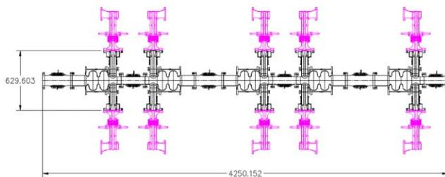
Figure 1: Cavity layout for Cornell ERL prototype injector.
