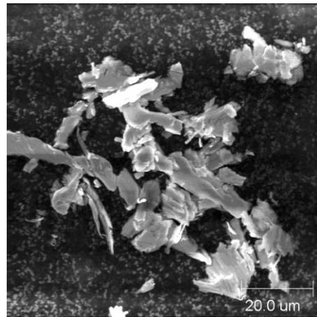
Figure 4: Copper particles generated from RF fingers.
