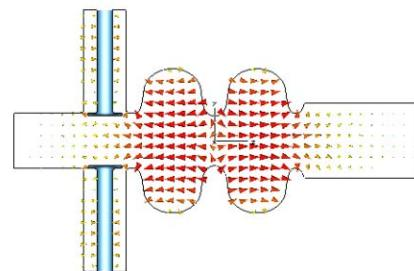
Figure 2: 2-cell cavity with twin RF input couplers.
