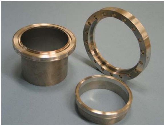
Figure 3: Conflat flanges for 2-cell niobium cavity. Left: vacuum furnace braze; Right: explosion bonding.
