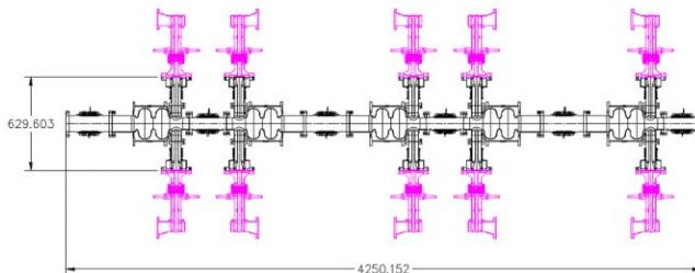
Figure 1: Cavity layout for Cornell ERL prototype injector.
