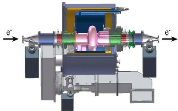
Figure 1: CESR-type cryomodule for TLS.
