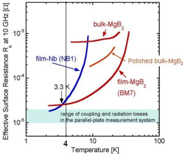
Figure 3: Surface resistance vs. temperature of a 400 nm MgB<sub>2</sub> film coated on a sapphire substrate. Bulk samples and Nb data are shown for comparison. [6]
