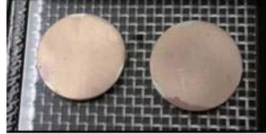
Figure 5: MgB<sub>2</sub> coated Nb disks of 14.6 mm in diameter.
