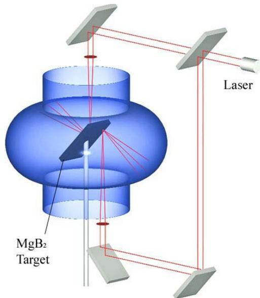
Figure 7: An idea for coating a cavity using a  $MgB_2$  target and a KrF excimer laser.
