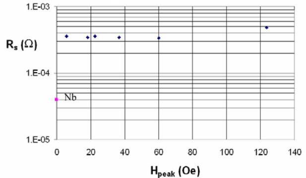
Figure 6: R<sub>s</sub> of the Nb TE<sub>011</sub> mode cavity with a MgB<sub>2</sub> sample at the center of the bottom plate, as a function of the peak magnetic field on the sample. The data was converted to 10 GHz using an f<sup>2</sup> law.
