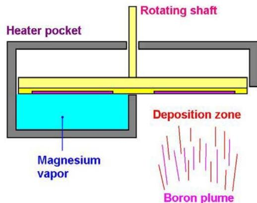
Figure 2: Cross section of the deposition chamber. [5]
