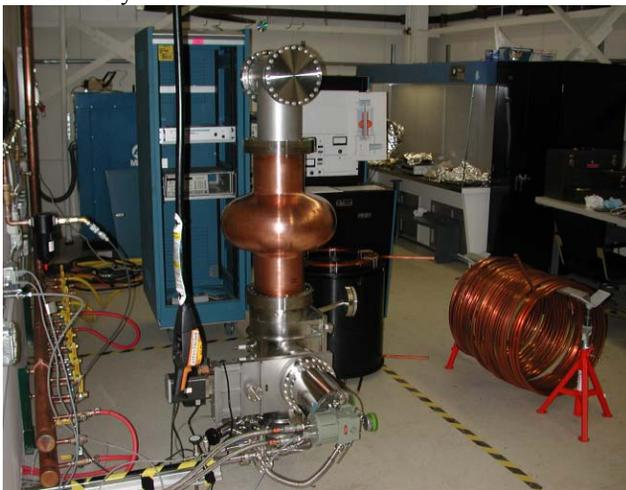
Figure 4: New thin film coating lab is being set up for 500MHz copper cavity deposition.
