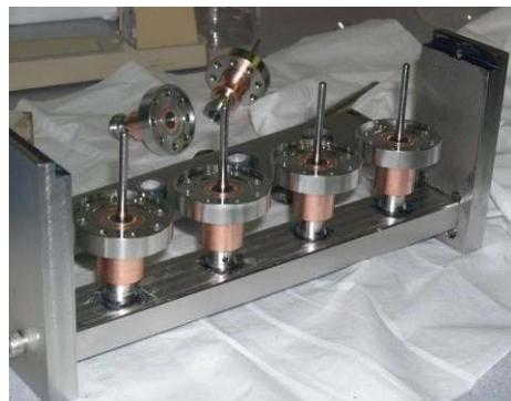
Figure 4. JLab single-crystal sapphire RF feedthroughs.
