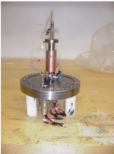
Figure 4: Thermal measurement set-up for measuring the heat transfer through the feedthrough into the He bath.
