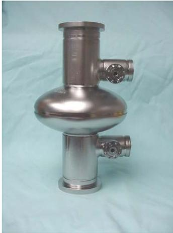
Figure 7: HOM Coupler Test cavity.
