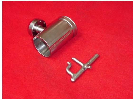
Figure 6: Modified HOM coupler loop
