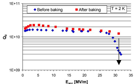
Figure 2: Performance of 1.5 GHz single cell cavity fabricated from ingot A niobium, before and after "in-situ" baking at 120  $^{\circ}\text{C}$  for 48 h.  $E_p/E_{\text{acc}} = 1.77$ ,  $B_p/E_{\text{acc}} = 4.47$  mT/(MV/m).
