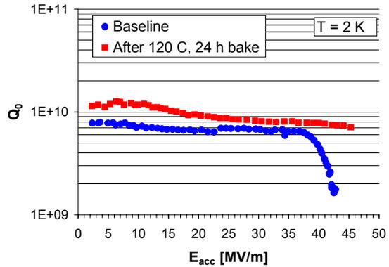
Figure 6: Test results from the LL\_ILC single crystal cavity.
