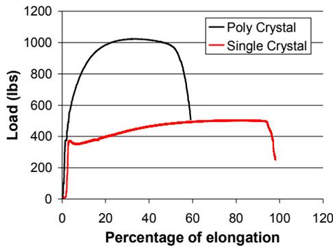
Figure 1: Load-elongation curves for the single and polycrystalline niobium samples.
