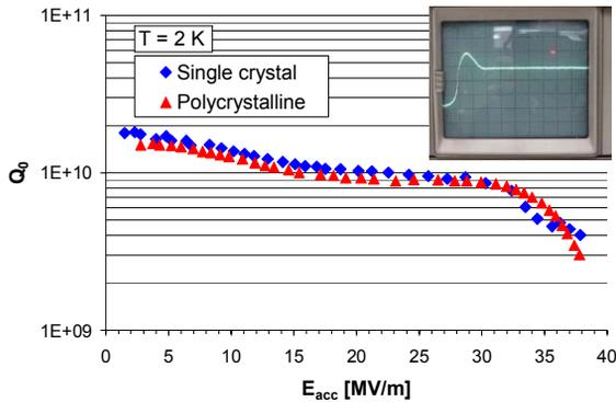
Figure 4: Performance of single crystal cavity from Figure 3 and identical polycrystalline cavity after “in situ” baking. As shown on the scope screen, the transmitted signal during the test of the single crystal cavity reached a value of 185 mT ( $E_{acc}=43$  MV/m), but leveled off at  $\sim 162$  mT after app. 300 msec.
