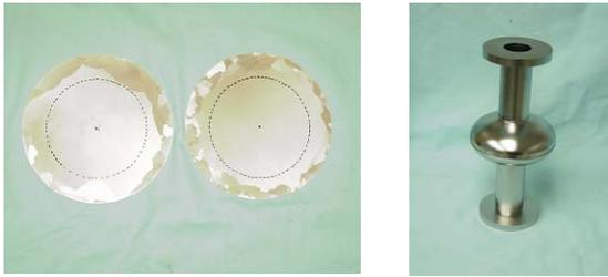
Figure 3: Single crystal niobium (ingot “A”) used to fabricate the 2.2 GHz cavity on the right side of the figure.
