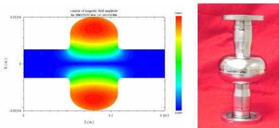
Figure 5: LL-ILC cavity shape with reduced surface magnetic field ratio:  $B_p / E_{acc} = 3.56$  mT/(MV/m),  $E_p/E_{acc}$  increased to 2.07.
