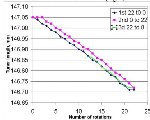
Figure 6: Blade tuner elongation measurement
