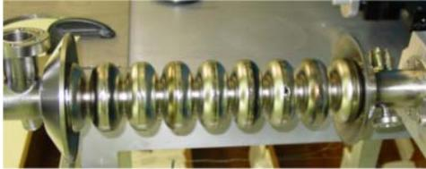
Figure 3: First 9-cell SRF cavity.
