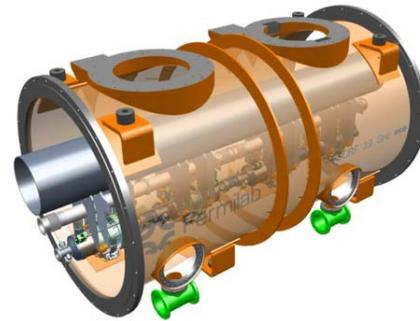
Figure 1: Cryomodule design for 4 cavities.
