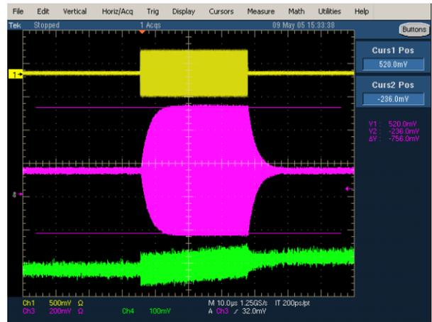
Figure 4: RF signals of the room temperature conditioning with 32μs, 2 kW pulses (forwarded power, resonator response and VCO-signal).
