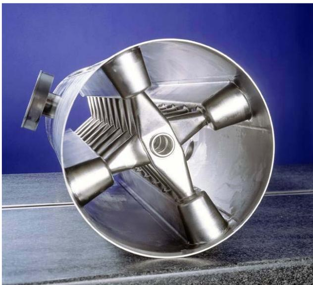
Figure 1: The superconducting CH-structure.
