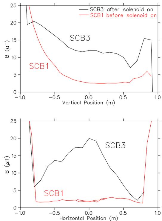
Figure 2: Longitudinal and vertical magnetic field maps inside cryomodule SCB3 (warm) after Test II compared to a mapping on new cryomodule SCB1.
