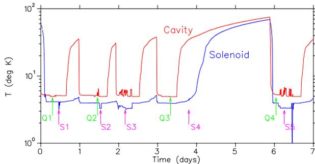
Figure 3: Temperature history of cavities and solenoid during Test-III. Q1-Q4 indicate the time of the  $Q_0$  measurements reported in Table 1 and S1-S5 indicate solenoid ‘on’ periods.
