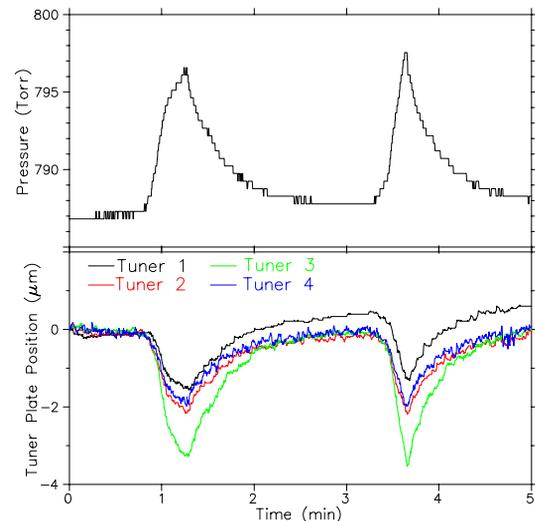
Figure 5: Tuner position response for forced pressure fluctuations in the helium space. The cavity gradient is 6 MV/m with a bandwidth of  $\pm 20$  Hz.
