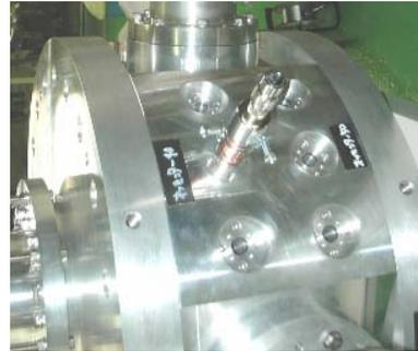
Figure 5: Al model cavity with off-centred damper
