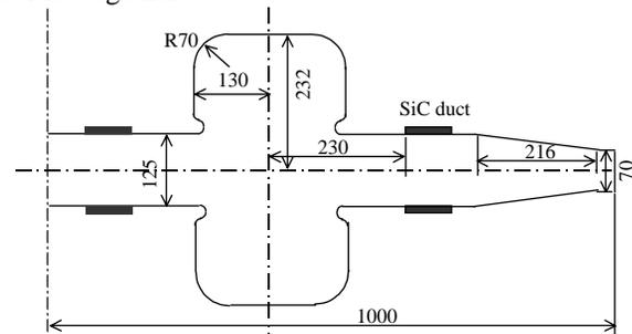
Figure 1:The cross sectional view for a half of 2 cavities
