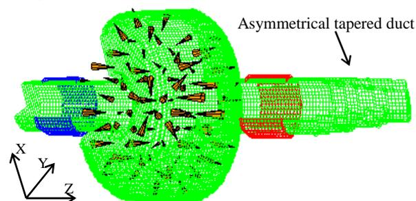
Figure 7: The 3-D electric field pattern (TM022-like mode)
