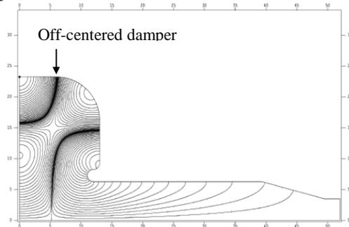
Figure 4: The example of the electric field pattern of HOM (Beam bore diameter 125 mm, TM022-like mode)
