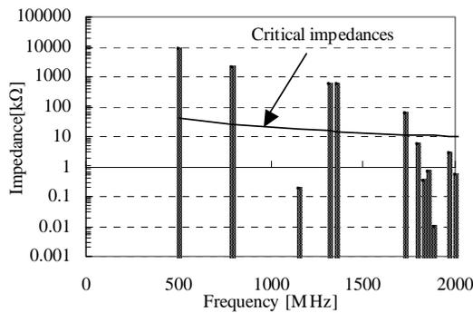
Figure 2: The longitudinal impedances of HOM's
