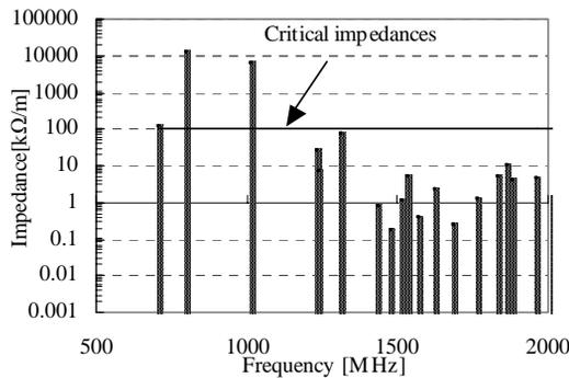
Figure 3: The transverse impedances of HOM's
