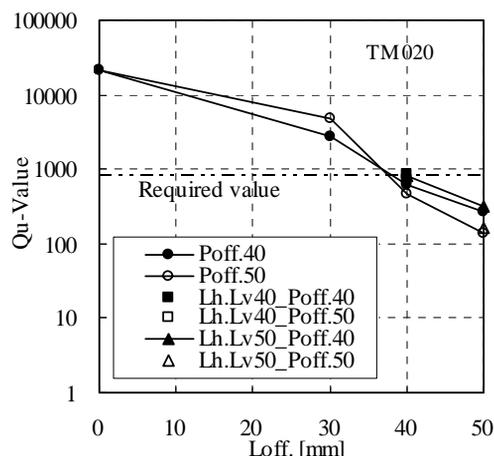
Figure 6: The antenna length of off-centred damper vs. HOM Q-Value
