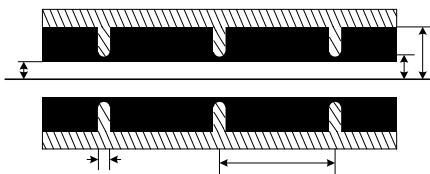
Figure 1: Schematic drawing of a hybrid dielectric-iris-loaded accelerating structure.
