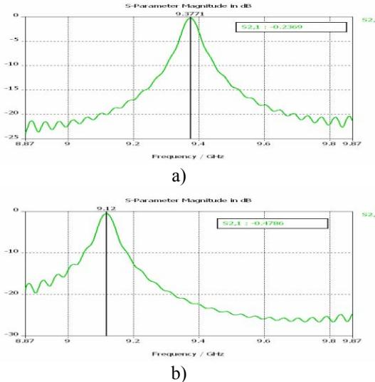
Figure 8: The simulation results of  $S_{21}$  vs frequency using the Microwave Studio. a) without the dielectric sample. b) with the dielectric sample
