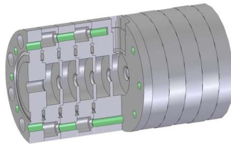
Figure 4: Cutaway drawing of the assembled 9-cell cavity design.
