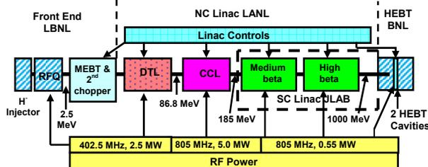
Figure 1: SNS Linac RF System.
